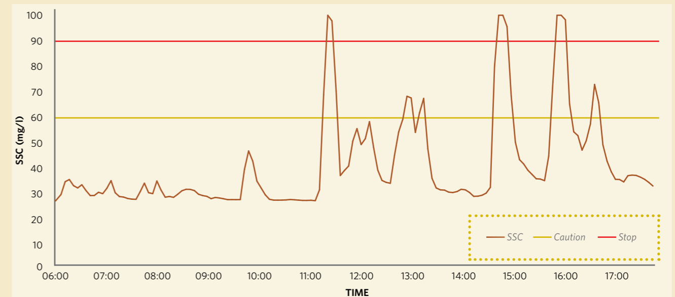
Figure 3.7: Example of SSC measurements and associated caution and stop trigger thresholds.
