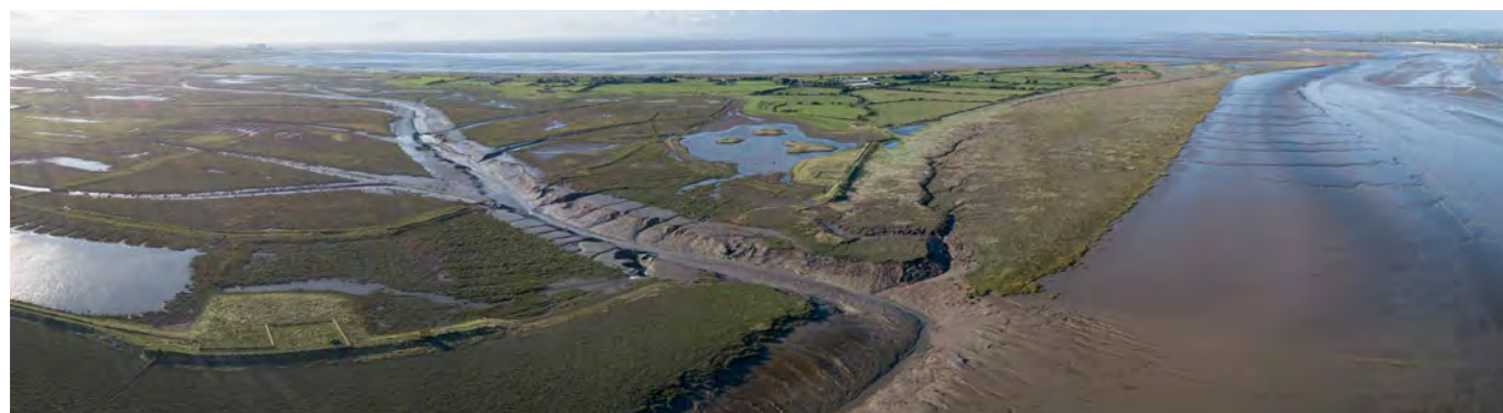
The 488 ha Steart Marshes managed realignment project on the River Parrett, Somerset, has restored 305 ha of intertidal habitat. Although managed realignment sites experience accretion following reconnection to the local estuarine and coastal system, in some instances, dredged material may be used to support land raising or landscaping and help reduce potential impacts on hydromorphology and geomorphology (Sam Stafford, Wildfowl and Wetlands Trust (WWT)).
